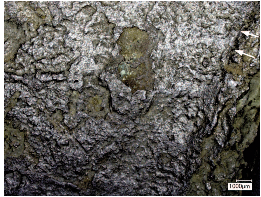
Fig. 6. Decoration visible as brighter reflections, indicated by the white arrows top right. The axe's edge faces upwards in this image. Photo from Keyence VHX-5000 by CH.
