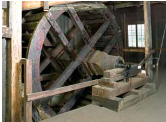
◀ All the technical equipment has been preserved complete with refining hearths and water-powered hammers. Photo: Bengt A Lundberg/Raä.
