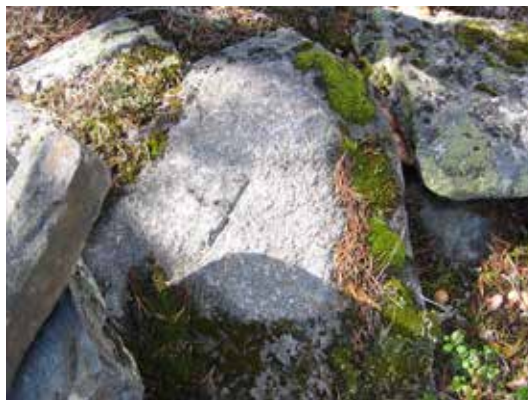
Perävaara triangulation station, part of the Struve Geodetic Arc, is marked with a cross engraved on a stone. Photo: © Dan Norin/Lantmäteriet.
