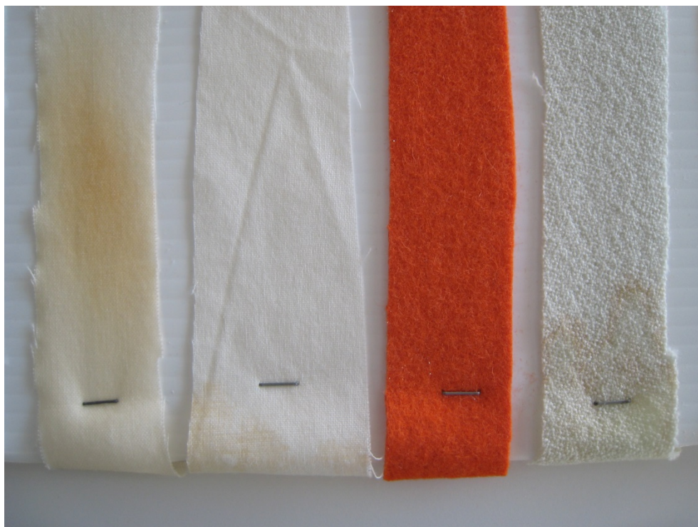
Figure 2. Samples exposed for one year placed vertically in window facing north. Effects of Secura (FR2) on test weave (to the left), orange fabric (1) and sand-coloured fabric (2). Salt migration can be seen in the lower part on test weave and fabric 2 (to the right). To the far left; brown discoloration on test weave sample treated with Apyrum (F1). Photo Margareta Bergstrand.
