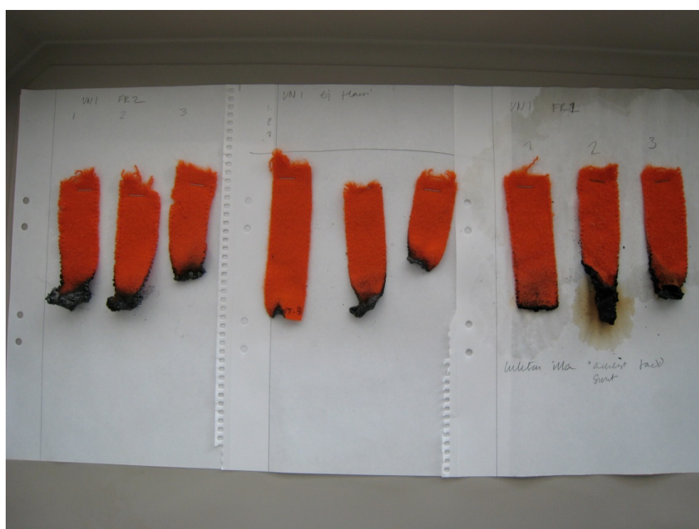
Figure 1. The untreated orange fabric UN1 (specimens in the middle) showed a better resistance to flammability than samples of the fabric treated with flame retardants Apyrum (FR1) to the right and Secura (FR2) to the left. Note the spots of moisture from Apyrum (FR 1). Photo Margareta Bergstrand.
