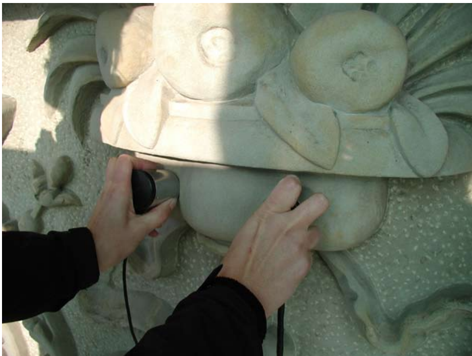
Figure 3. Ultrasonic measurements undertaken at the German Church.
