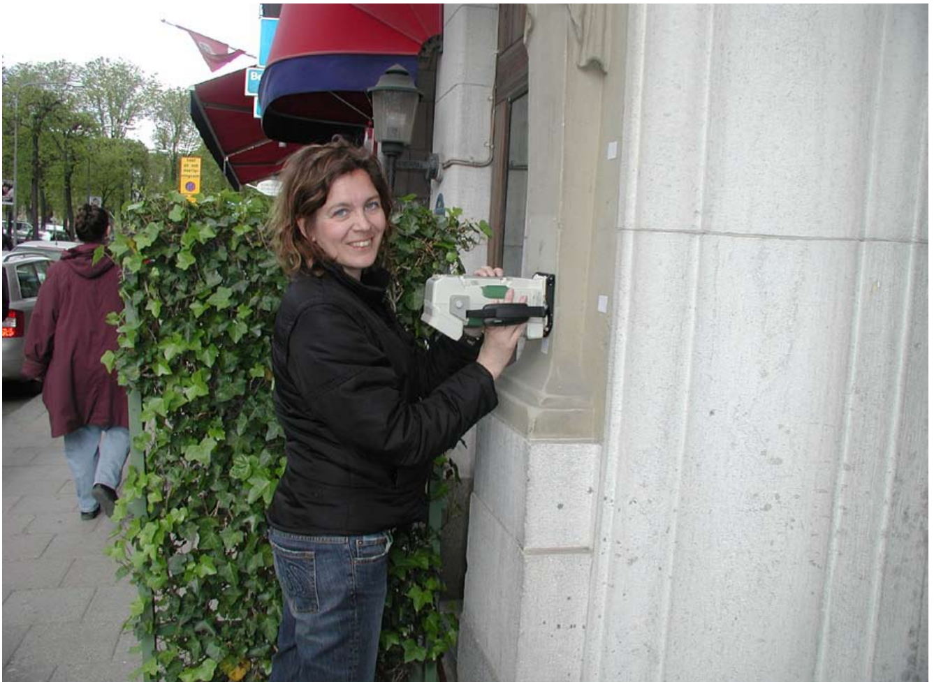
Figure 5. Colour measurements using a Minolta CM-508i at Narvavägen 30.
