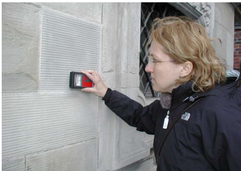
Figure 4. Moisture measurement with a Tramex at Karolin Chapel.
