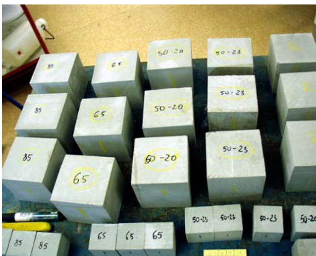
Figure 1: Samples used for the UPV analyses. Markings on the samples indicate the relative humidity.
