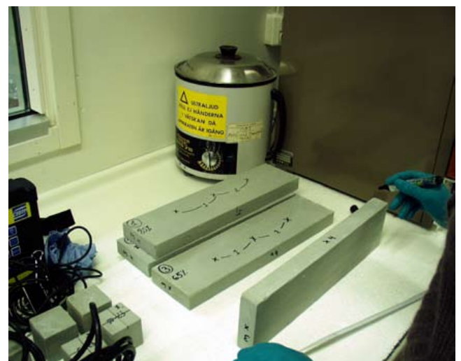
Figure 1: Samples used for the UPV analyses. Markings on the samples indicate the relative humidity.
