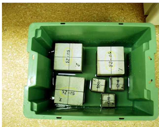
Figure 2: Water absorption test.
