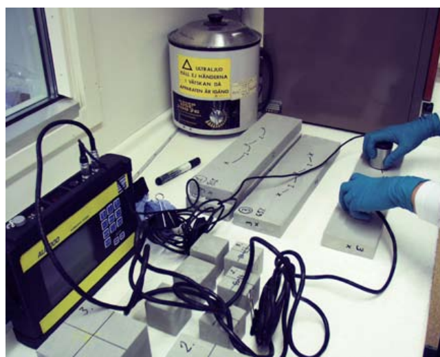
Figure 3: Indirect measurement of UPV.
