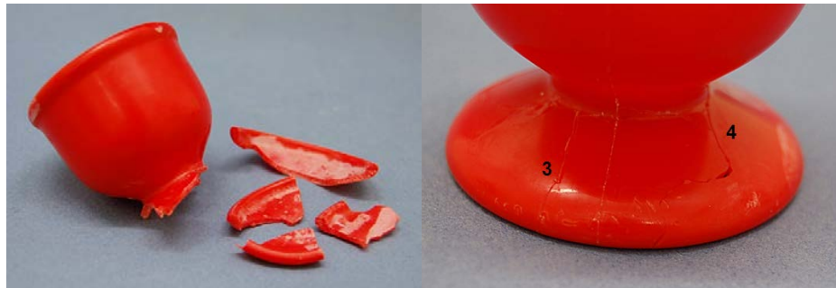
Figure 38. Bond of Primal AC35 (3), and Hxtal NYL-1 (4).
