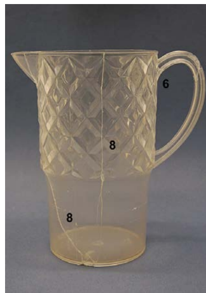
Figure 33. Bonds of Paraloid B72 in ethanol (8), Loctite SAP (6) and Hxtal NYL-1(4).
