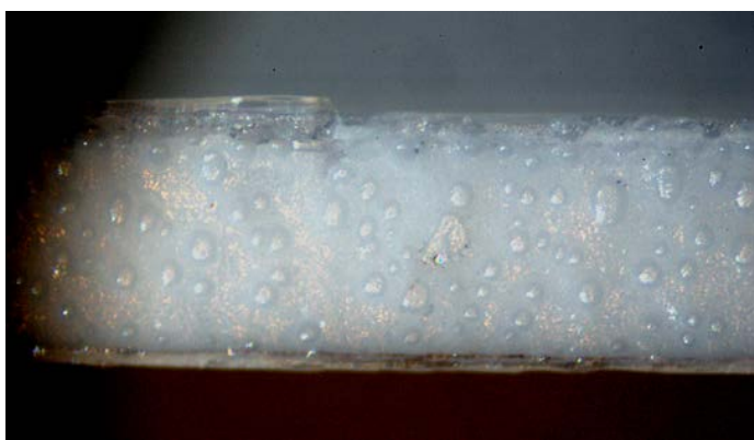
Figure 22. Sample H7 (Acrifix 116) unaged in regular microscope. Example of cohesive break in the adhesive.
