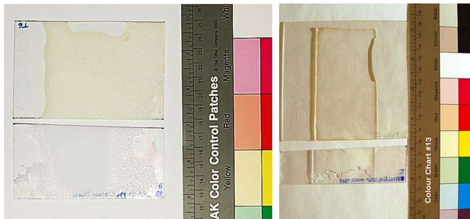
Figure 11. Loctite SAP (left) and Araldite 2020 (right) on transparent polystyrene before (bottom) and after (top) ageing.
