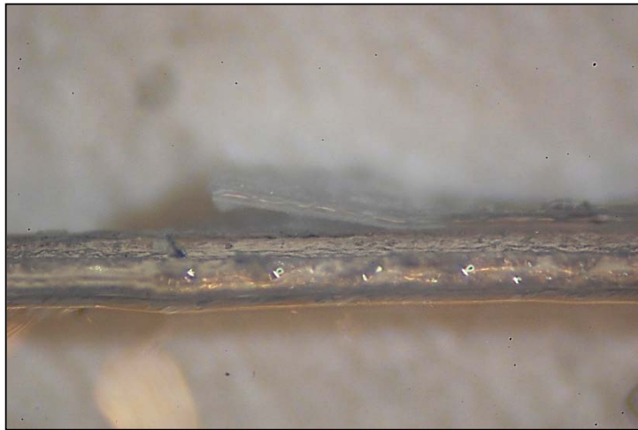
Figure 20. Epoxy loosened from S1.
