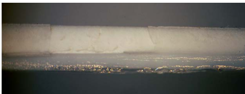
Figure 21. Sample H4 (Hxtal NYL-1) unaged in regular microscope. Example of adhesive break.
