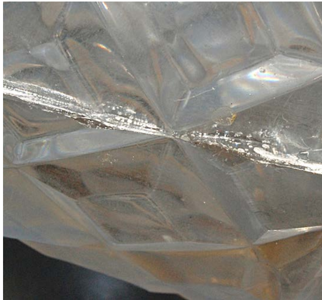
Figure 36. Bond of Paraloid B72 in ethanol
