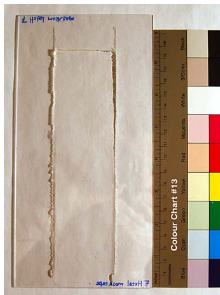
Figure 6. Example of Hxtal-Nyl 1 on transparent GPPS before ageing and before cutting.
